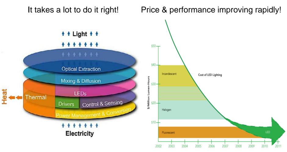
Cost of Light includes: lifetime, source efficiency, energy cost, replacement cost of lamp/fixture, labor cost
